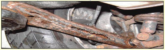
This picture shows what a radius arm can look like after my pressure wash. This car belongs to John Hudson in High Wycombe. Before I pressure washed the radius arm there were no apparent holes in it. Yet as you can see from the picture it was actually so corroded that he was actually putting himself and other people in danger driving the car. I would like to make 2 points here:
