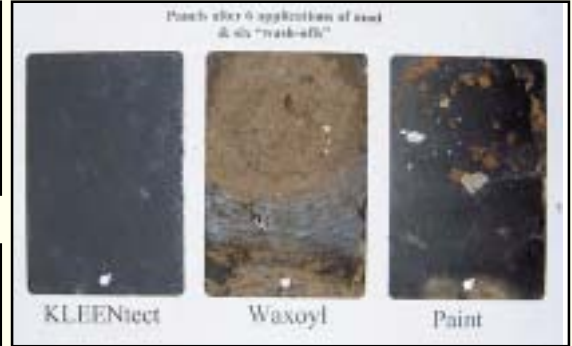
Test plates show: KLEENtect, Waxoyl and painted panels. Mud was applied, allowed to dry then washed off 6 times: After 6 th wash off, KLEENtect panel is perfect and retains high gloss with no abrasion damage whatsoever. See videos of these tests on www.before-n-after.co.uk . Test continues.....
